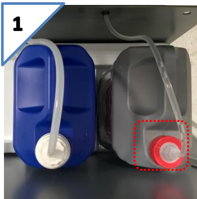
1 Disconnect the connector from the can
